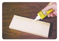
**5.** Apply a bead of leathercraft cement to the other two lines as shown.
