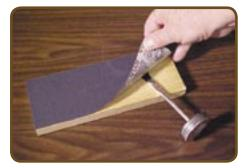
**1.** Attach a piece of 600 Grit Wet/Dry sandpaper to one side of the block as shown.
