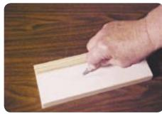
Make your own versatile stropping block with a piece of  $1'' \ge 4''$  lumber, a sheet of 600 grit wet/dry paper, a piece of thin leather, a piece of 2mm leather lace and a 1/8'' strip of 8/9 oz. Cowhide. Works great for sharpening and honing all knives, especially hard to sharpen edge bevelers.
