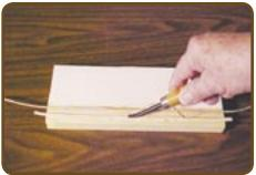
**6.** Cement 2mm round leather lace and 1/8" leather strip to block. Allow cement to dry and trim both edges of 1/8" strip with a #3 edge beveler.
